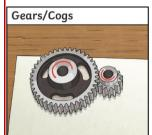
Gears or cogs can be used to change the speed, force or direction of a motion.
