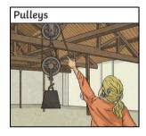
more wheels in a pulley, the less force is needed to lift a weight.
